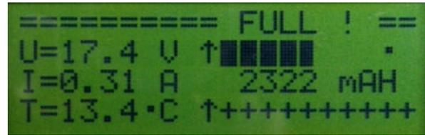
The charging continues till the moment when the batteries reach their maximum capacity which also reflects in increase in the temperature. When reaching their full capacity and increase in the temperature up to 40°C the charging stops and down on the display you will see “FULL”. At the same time the device will start to make short sound signals.
